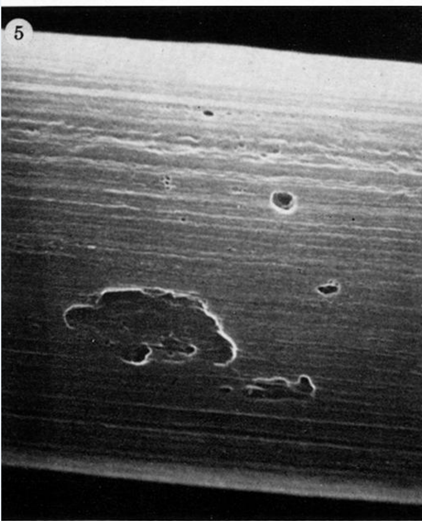
FIGURE 5. Surface defects on carbon fibre.
